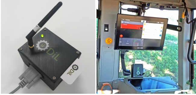
Fig. 3. Prototypical realization of the developed AML using NFC cards for a continuous user authentication on agricultural machines.
