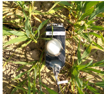
(b) Sensor node deployed in the wheat field.
