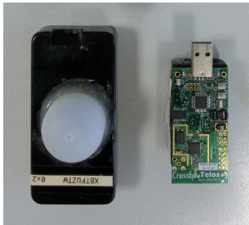
(a) TelosB and the enclosure with a diffuser cap for its PAR sensor.
