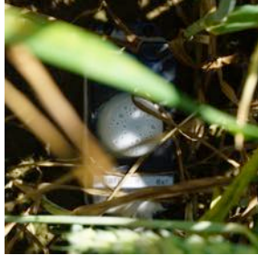
(a) Condensation water under the diffuser cap of sensor 0x7 (DOY 178).
