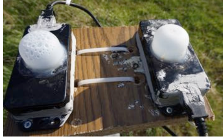
(b) Condensation water under the diffuser cap of reference sensor 0xB and traces of bird droppings (DOY 125).
