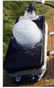
(a) Condensation water in the diffuser cap of a PAR sensor.
