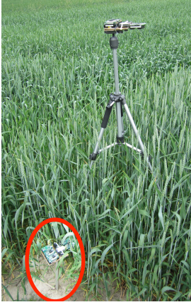
(a) Pair setting with one TelosB on a tripod above and a second one below the canopy (red ellipse) deployed in a wheat field.
