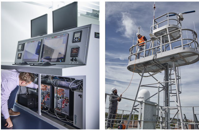
Fig. 2. INS with real antennas and hardware systems, installed in accordance with classification rules and behaving as a real ship bridge.
