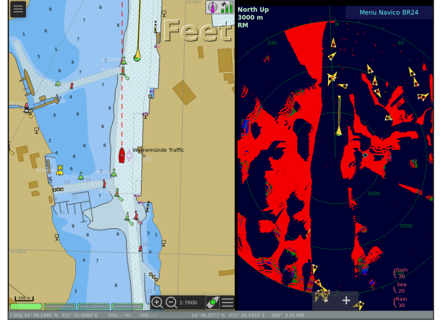
(b) The surroundings can still be perceived through AIS and radar information visualized by OpenCPN 's radar_pi plugin.
